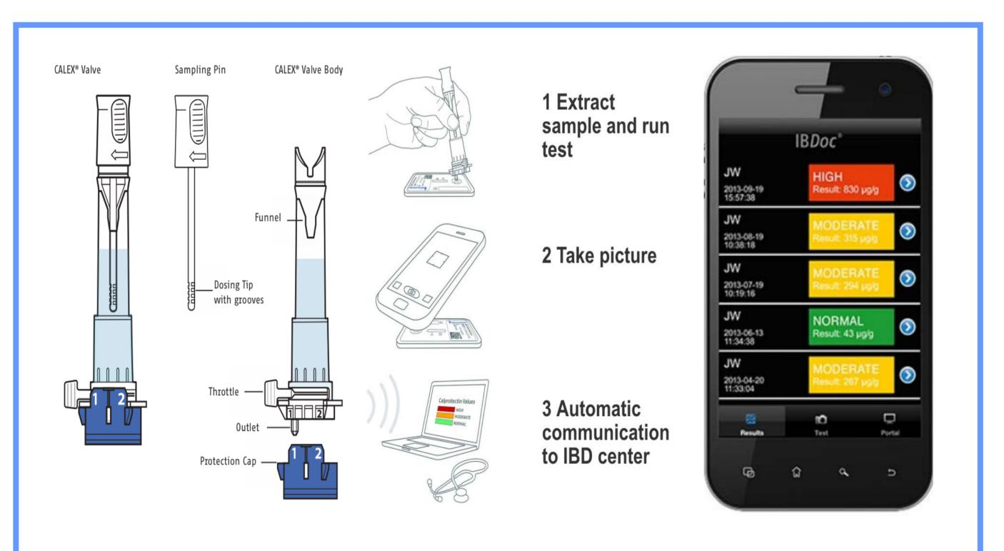
**Figure 1.** Components and schematic of the IBDoc™ test. The proprietary Calex™ valve tube is used to collect and prepare a sample for analysis. A predetermined volume is applied to a calibrated test reading strip which is imaged by the App, generating a result which is communicated immediately via web portal to the team.
