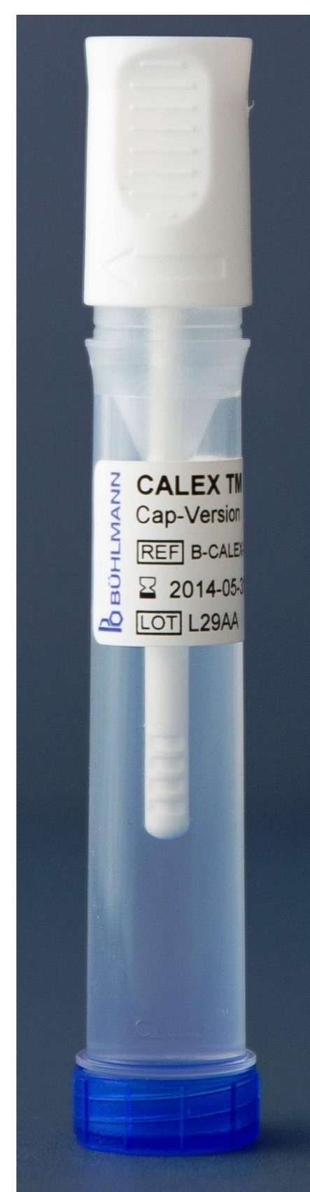
Fig. 1: CALEX ® Cap device consisting of white sampling pin with grooves at its tip, transparent body with funnel (filled with extraction buffer to provide an extractive dilution of 1:500), and blue screw cap.
